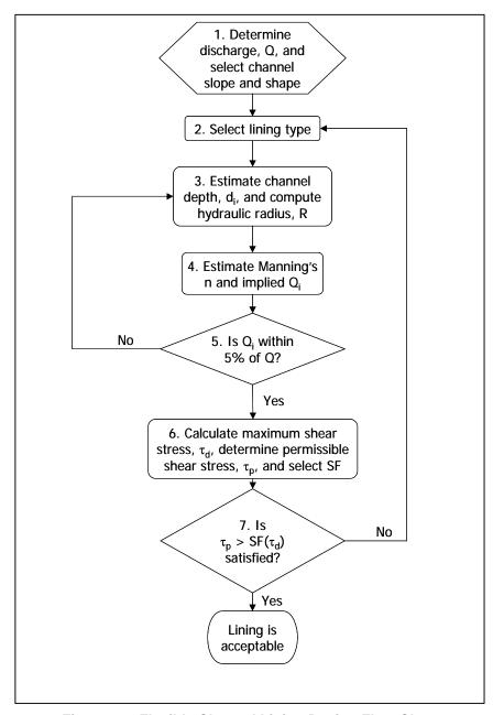
Figure 3.1. Flexible Channel Lining Design Flow Chart
