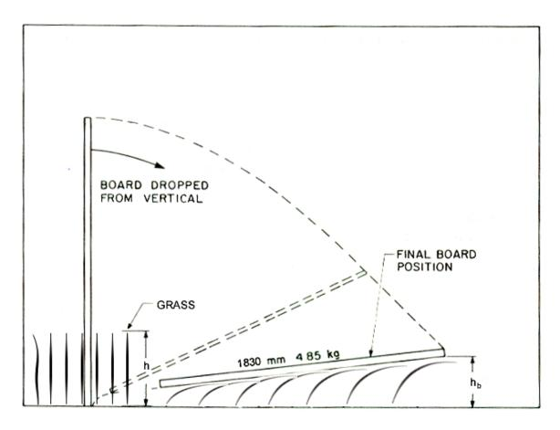
Figure E.1. Schematic of the Fall-board Test (after Kouwen, 1988)
