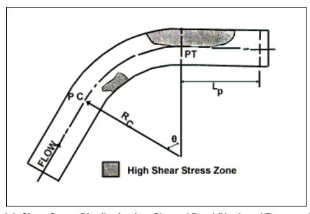
Figure 3.3. Shear Stress Distribution in a Channel Bend (Nouh and Townsend, 1979)
