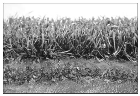
Figure 1.7. TRM Profile with Vegetation/Soil/TRM Matrix (Source: ECTC)
