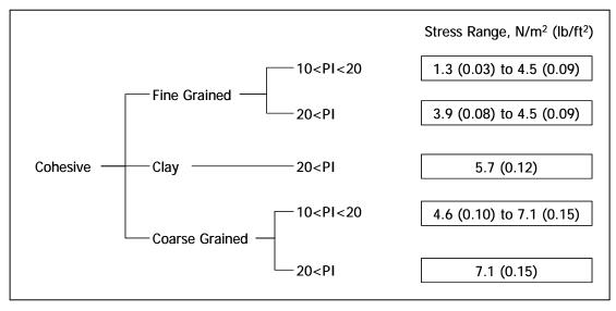
Figure 4.1. Cohesive Soil Permissible Shear Stress
