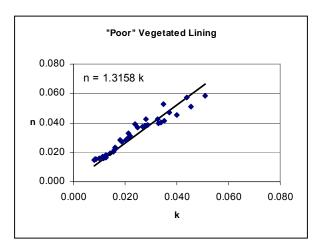
Figure C.1c. Relative Roughness Relationships for Poor Vegetated Conditions
