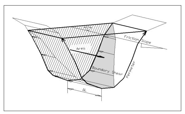
Figure 2.1. Typical Distribution of Shear Stress
