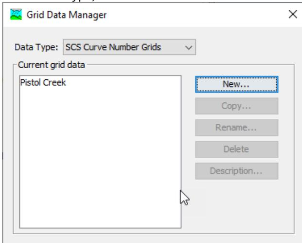
Once you click OK, the SCS Curve Number Grids folder will appear under the Grid Data folder. Expand the SCS Curve Number Grids and select Pistol Creek. In the Component Editor, navigate to the location of your DSS file in the data folder (or wherever you saved your DSS file with the CN grid). In the DSS Pathname, select your CN grid record and save the project. In the Component editor of your subbasin element, select the CN grid in the loss tab.
