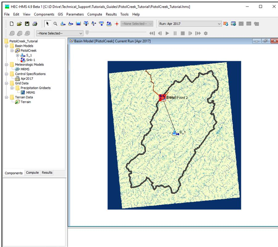
Under the Basin Model, select Pistol Creek basin model. Check through all of the methods and parameters. You'll notice that all of the methods and parameters have already been provided except for the Loss Method. Under the Loss Method, select **Gridded SCS Curve Number**.
