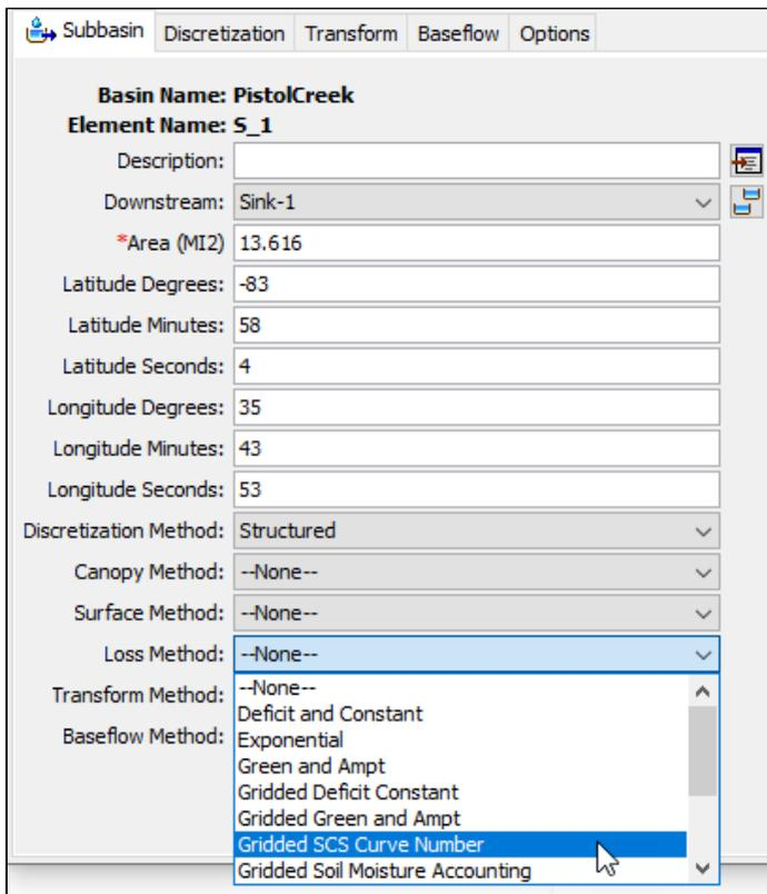
In the Discretization tab, make sure the Projection and cell size is set to **SHG** and **50** meters. These values should be familiar to you since we set them during the CN grid import process. In the GIS menu, select Compute → Grid Cells to create your Discretization grid layer. You can view the created layer in the View → Map Layers editor. Make sure you check "Discretization".
