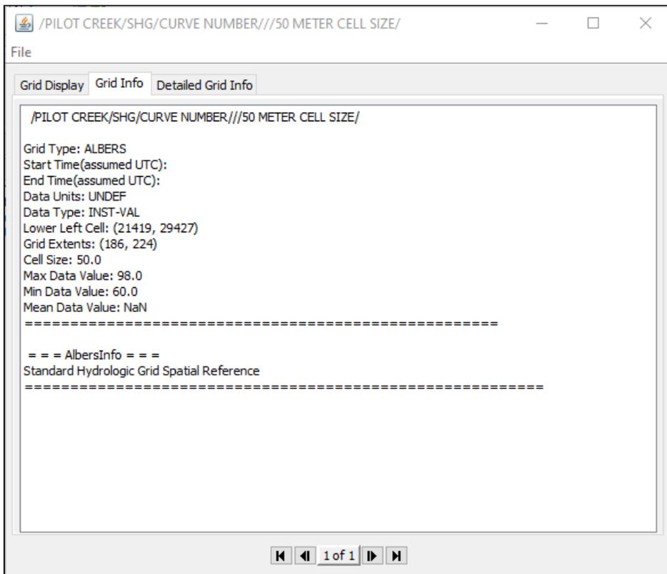
Once those are confirmed, you will need to rename the Part C of the DSS record to **CURVE NUMBER**. This lets HEC-HMS know this grid is a curve number grid. Once these are checked, you are ready to import the grid into HEC-HMS.
