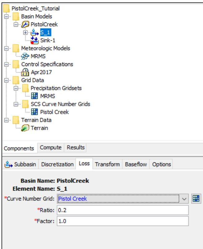
Check that the CN grids were set up correctly by running a simulation. Head over to the compute tab and run the Apr 2017 simulation. The simulation should run to completion.
